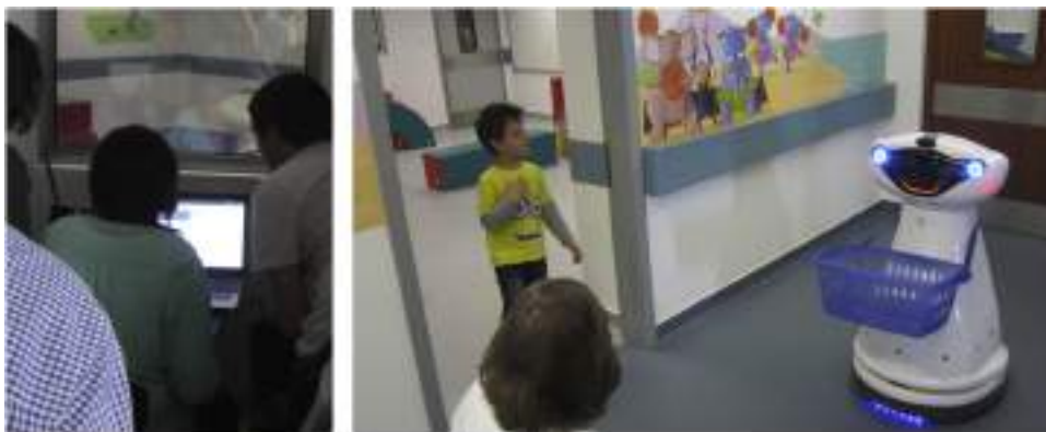
Fig. 13. Illustration of the preliminary studies. Left: Two wizards control the robot behavior—the operator in front of the computer controls the interaction, while the one standing navigates the robot. The robot top is visible on the one-sided mirror in the background. Right: Therapist mediated interaction at the end of a therapy session. The child brings the robot to the door to say goodbye. Visible in the background is the room where the interaction took place.
