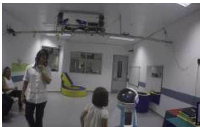
Fig. 8. Example of a task specific behavior of the robot. Upon detecting an obstacle, ASTRO makes a sad face and tries to find a way around, before asking the child for assistance. In the background it is visible the whole hardware infrastructure of INSIDE.
