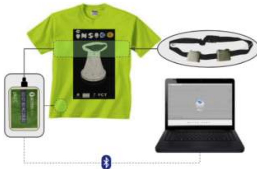
Fig. 15. T-shirt designed to collect physiological signals from the children interacting with the robot. The T-shirt comprises a chest-band and an acquisition module. The chest band is located near the diaphragm of the user, while the module is placed in a small pocket, on the down right position of the T-shirt.
