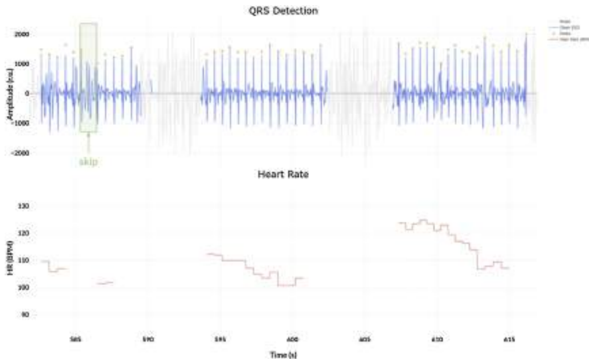
Fig. 16. Heart Rate determination in the areas of clean ECG. The areas that are not represented in the Heart Rate plot are either noise or false peak detections.
